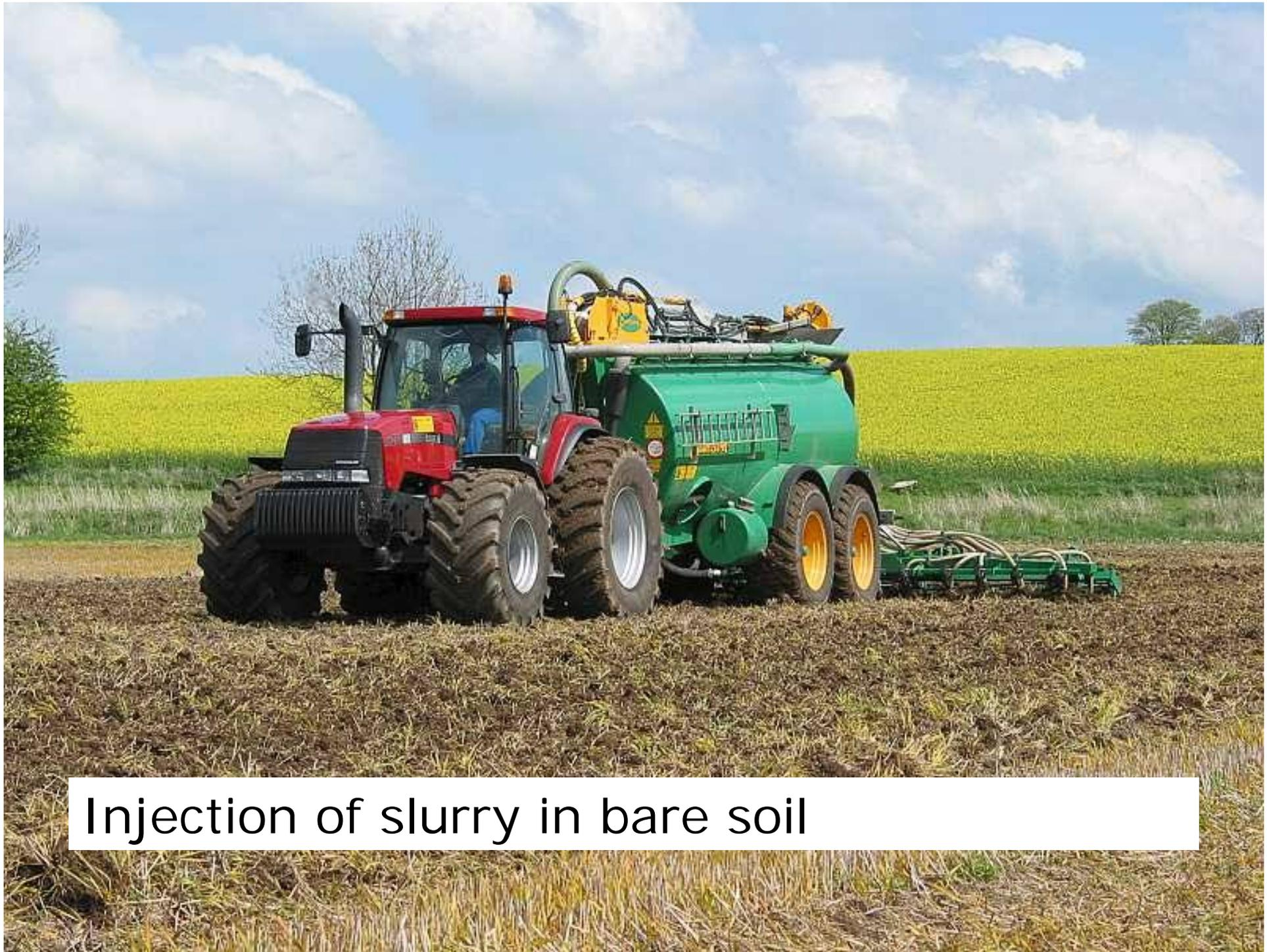
Injection of slurry in bare soil
