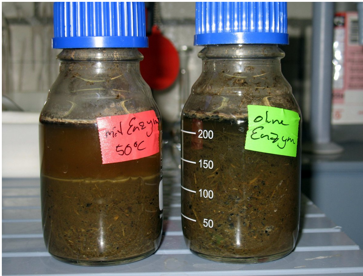
Fig. 1: Grass silage incubated with and without hydrolytic enzymes (cellulase + hemicellulases) for 15 h at 50 °C.
