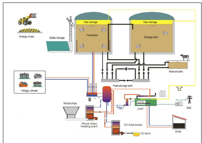
Figure 2: Schematic draw of the bioenergy plant Jühnde
