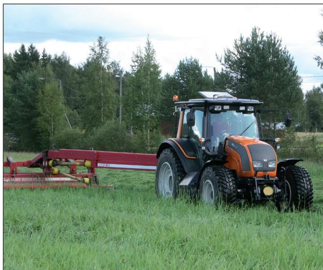
Figure 4. Valtra dual-fuel biogas tractor in test use on the Kalmari farm (Metener Ltd.)
